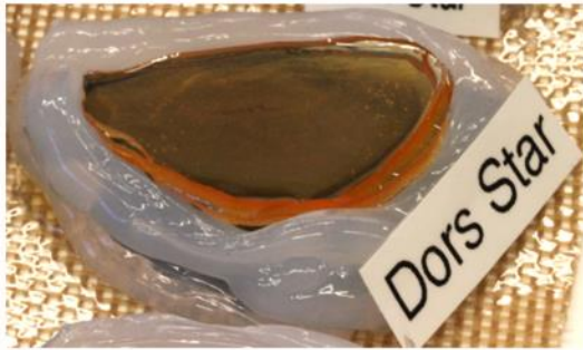
Supplementary Figure 5: Casting process. (a) Silicone mold with ridges. (b) Molds are labeled and lips are made so that molds can be cast. (c) Mold casted in two-part epoxy resin. (d) Mold removed and ready for surface profilometry.
