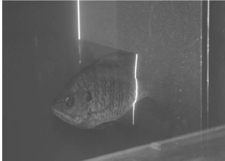
Fig. 6. Bluegill sunfish swimming in a flow tank that has been seeded with small reflective particles. Light from an argon-ion laser has been focused into a light sheet and projected into the tank to intercept the body of the sunfish transversely. The pectoral fin is beating upstream of the light sheet, and free-stream flow in the tank is from left to right. Flow from the pectoral fin travels downstream and through the light sheet, and is imaged with cameras located downstream of the light sheet that are viewing the flow coming toward the camera sensors.
