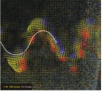
quantified this aspect of foil locomotor dynamics using the volumetric flow visualization system described by Flammang et al. (2011a, 2011b) and Troolin and Longmire (2010). Figure 5 shows how each of the centers
