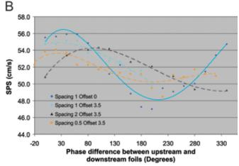
as the distance between the foils is increased the peak swimming speed shifts toward a larger phase lag of the downstream foil. Interestingly, the maximal swimming speed of the two foils together does not change significantly as the distance between foils changes, and alterations in phasing between the foils can thus be used to compensate for changes in spacing.
